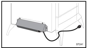
Fig. 13 Correct position of fan skirt installation.
